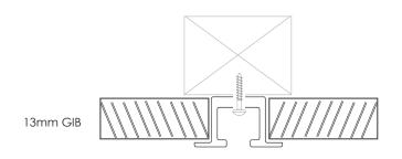
Flush Fit Track is a track recessed into the ceiling. The track sits inside the ceiling lining and requires no brackets for installation. Flush Fit track is 13mm high which is the standard thickness of ceiling lining sheet used in New Zealand (GIB) and Australia (Gyprock).
